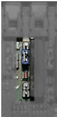
Jumper setting for relay output.
