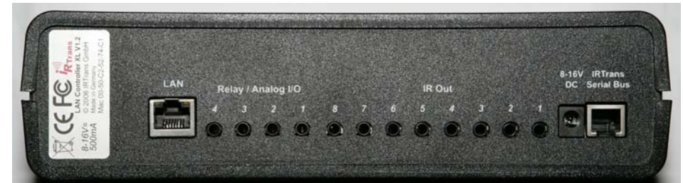
Back of the IRTrans LAN Controller XL
